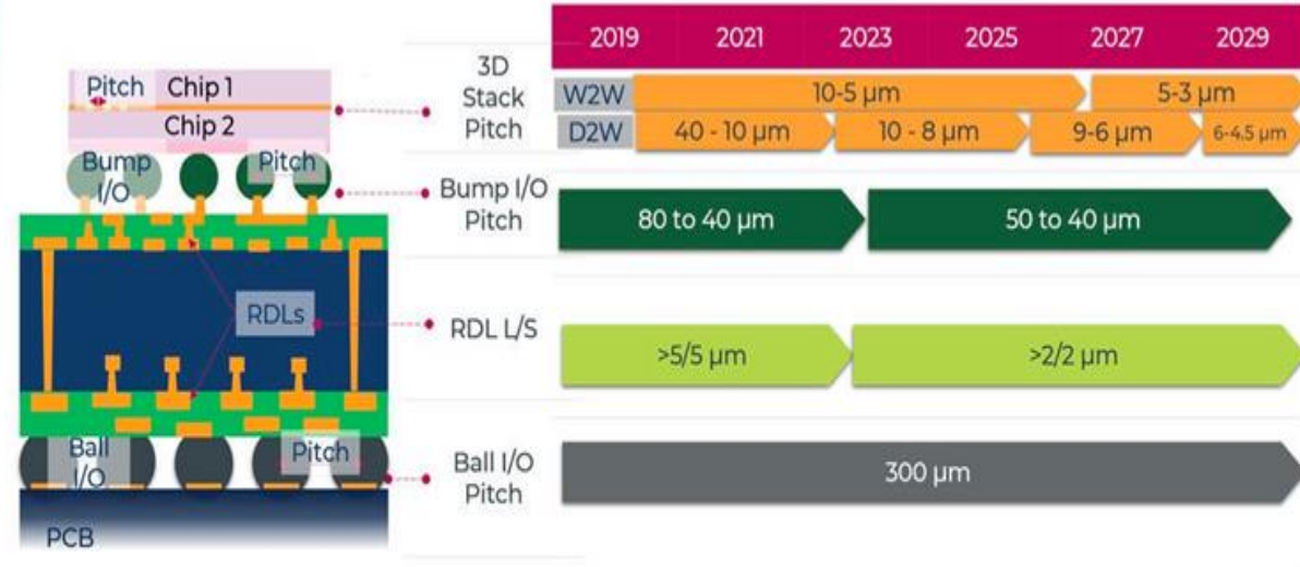
Advanced Packaging Roadmap -IO pitch & RDL L/S
